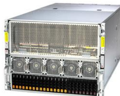
Figure 1 - 8U 8-GPU Server with AMD Instinct MI300X Accelerators
