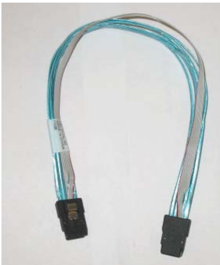
Figure 3-7: iPass (Mini-SAS) to iPass (Mini-SAS) (CBL-0110L-2)
